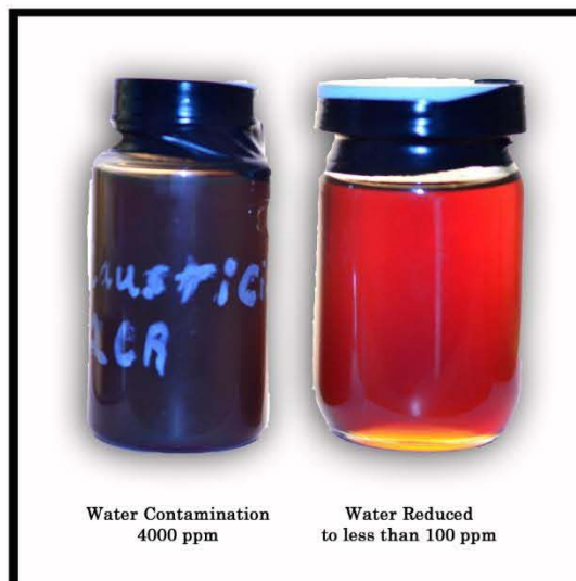
Paper Plant - field results 220 weight Gear Box Oil - 48 gallon reservoir
